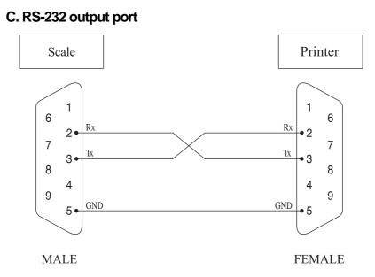
Connect EC-II and Printer using same cable. [male(EC-II) - female(DLP-50)]
