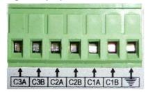
There are three section controllers, (C1A, C1B), (C2A, C2B), (C3A, C3B), Each of them has two wire connectors. They work respectively. The signal output port can be connected to a lamp, beeper, annunciator, etc. Note : (C1A, C1B)= LO, (C2A, C2B)=OK, (C3A, C3B)=HI
