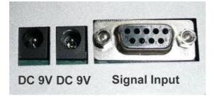
Use our standard cable to connect the signal input port with the scale or other equipment. And these two ports for power adaptor must be connected to make sure the control box is workable.
