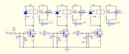
When it is connected with 3 color Annunciator, please use a cable to parallel C1A, C2A and C3A.
